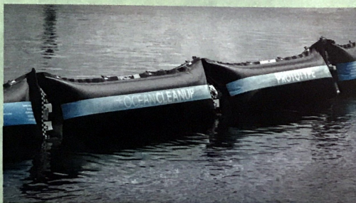
Figure 6.28 A prototype floating barrier designed to capture plastic waste
