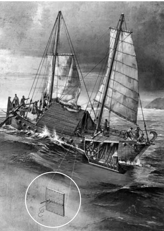
A trading dhow, showing how the side planks were stitched together to be watertight
