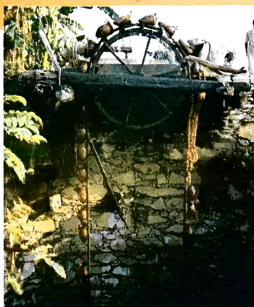
▲ Figure 6 A sakia or waterwheel. Oxen turn the wheel and cowhide buckets are lifted and emptied into field ditches.
